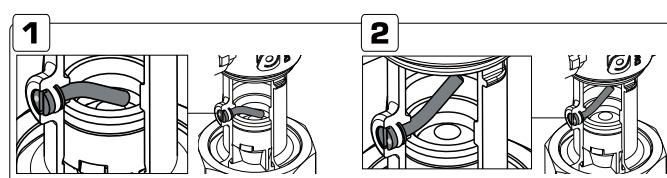
After a complete filling and venting, turn the screw on the check valve back to its normal operating position, picture 2 and set the circulation pump operation to recommended position.
